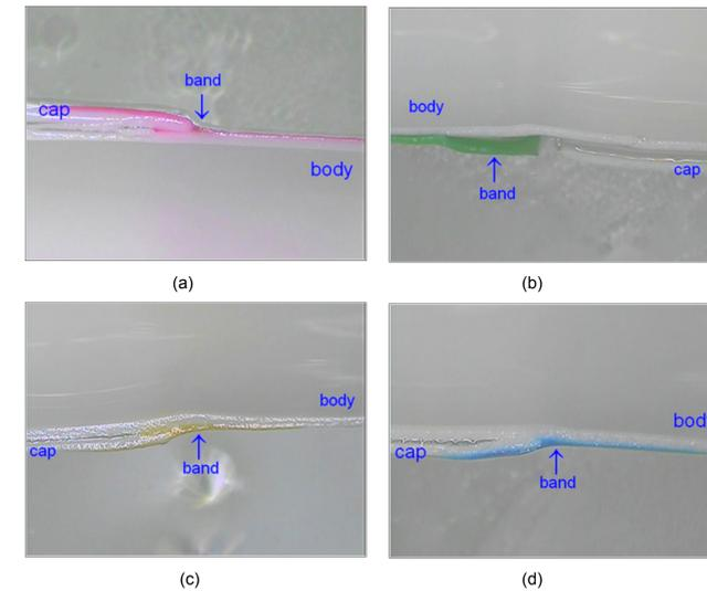
Figure 2. Cross-section of capsule banded area under microscope. (a) 16% HPMC and ethanol alcohol/water. (b) 22% gelatin water solution. (c) 22% HPMC water solution (d) 11% HPMC water solution with gelling agents.
