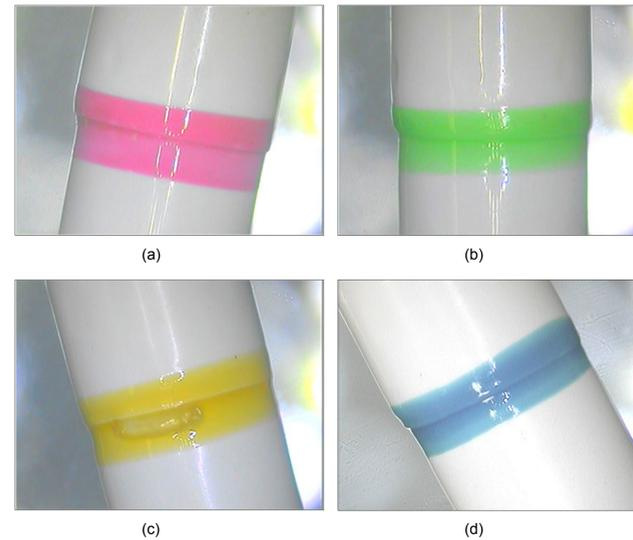
Figure 1. Banded capsules under microscope. (a) 16% HPMC and ethanol alcohol/water. (b) 22% gelatin water solution. (c) 22% HPMC water solution (d) 11% HPMC water solution with gelling agents.
